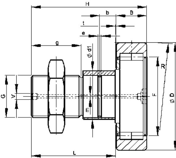
FSG cam rollers are comprised of a solid, collar stud, a thick-walled outer ring, and a full-rolled, rolling body component. Similar to the construction of cylinder, roller bearings; the thick-walled outside ring is positioned over the rolling body. Due to the thick-walled outer ring, these curved rollers are especially suitable for sustaining increased, radial loads.
