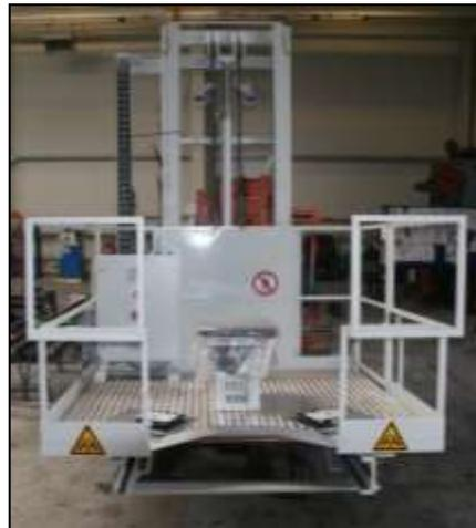
**Lifting platform with floor mounting and adjustable recess for spiral machining**
