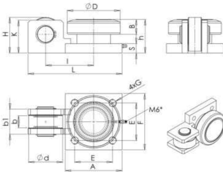
FSG axial roller skids absorb high forces on the radial and axial rollers and are well suited for use in harsh environments.
