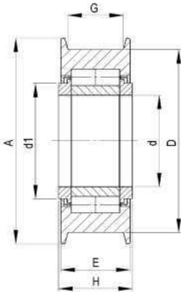
Chain pulley's get as well used at machinery and forklift trucks. The pull chains are turned around the chain rollers, which are fixed on the lifting cylinder or internal mast. Depending on the lifting gear construction, the wrap-around may be up to 180°. The requirements for the rollers depends on the number of the chains, the wrap-around angle as well as the load capacity of the machine.
