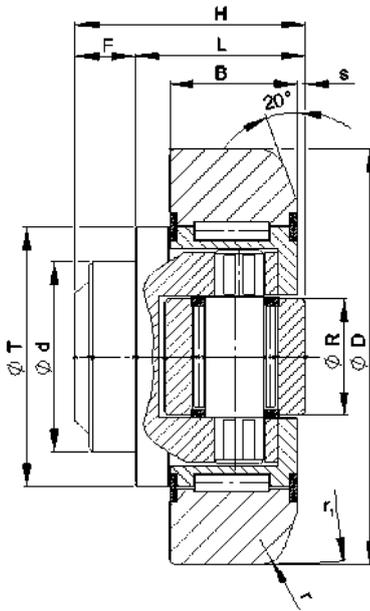
The axial roller is revealed by removing the front cover. By turning the axle, dimension H, L and s can be adjusted between 1.5 mm and 4.0 mm, depending on the size of the roller.
