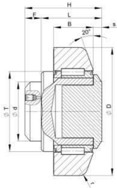
Distance plates can change the dimension H, L and s by up to 2.5 m. **Distance plates are included in the scope of the delivery. Per roller, 2 x 1 mm, 1 x 0,5 mm.**
