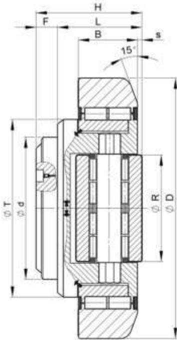
By turning the axle of the axial roller, the dimension H, L and s can be changed by up to 4 mm, depending on the size of the roller.
