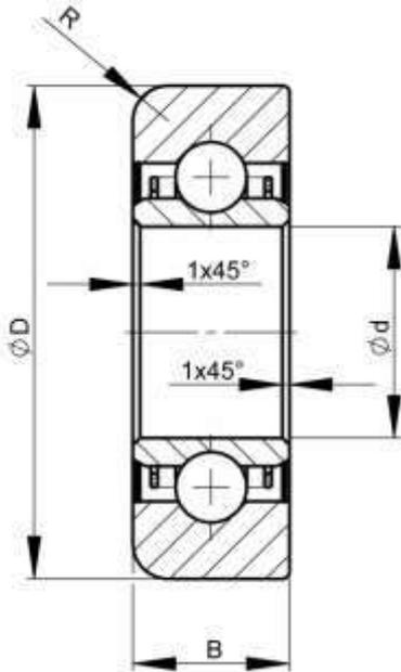
Our radial rollers with ball bearings are manufactured in accordance with DIN620 and are particularly suitable for light loads. The outer ring made from tempered steel can be used in both **U** and **I** profiles (see table).
