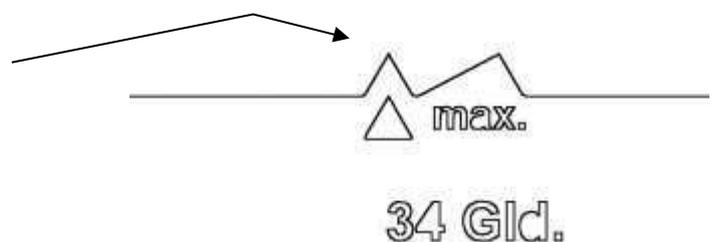
The chain lineal from FSG simultaneously includes the wear limit (refer to maximum)
