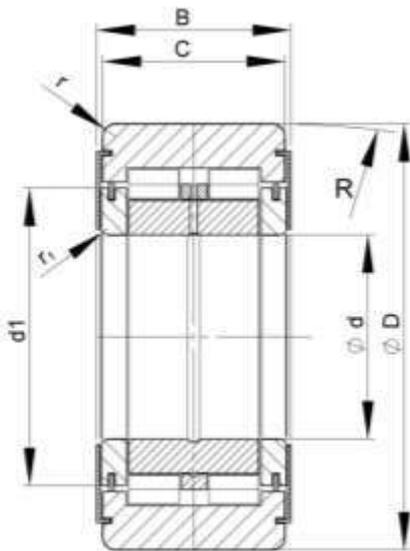
Support rollers are single or double-rowed, massive components which are mounted on axles. They consist of outer and inner rings and rib-guided, cylindrical rollers.
