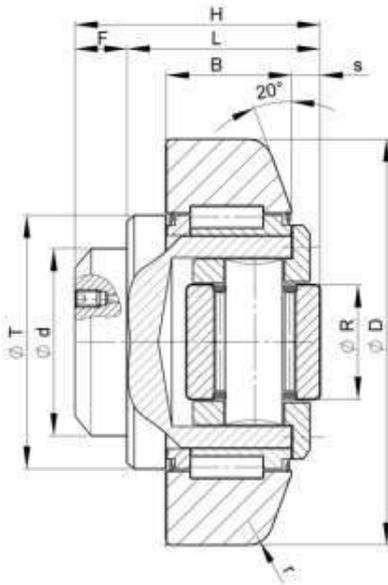
Distance plates can change the dimension H, L and s by up to 2.5 mm. **Distance plates are included in the scope of the delivery. Per roller, 2 x 1 mm, 1 x 0,5 mm.**
