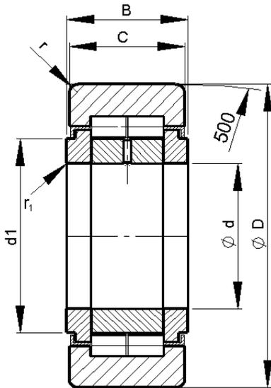
STG-rollers have a high radial load capacity in the radial area. To be also able to absorb and support axial loads, the inner ring and board ring must be tensioned. For example, by utilising a washer and locking ring or washer and nut.
