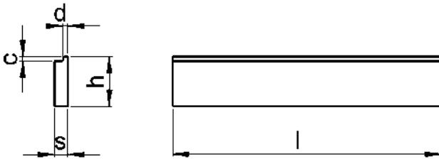
Fork carrier profile beading, hot rolled from S355J2G3
